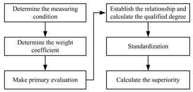
Figure 4. Specific steps of the Superiority Evaluation Method
